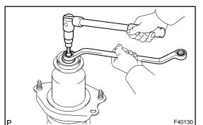
(e) Use a socket hexagon wrench (6 mm) to fix the shock absorber assy piston rod and tighten the nut.
