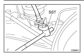
(c) Fully tighten the rear brake tube using SST.
