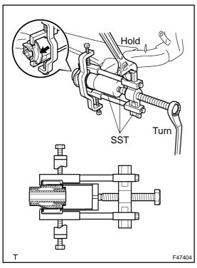
(c) Install the bush to the rear axle beam using SST.
