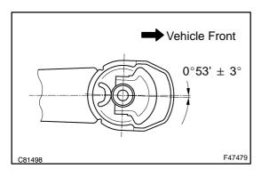
(b) Temporarily install a new bush as shown in the illustration (when replacing the rear axle beam).
