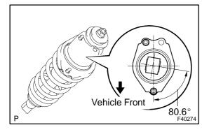
(d) Install rear spring bumper No.1, the rear suspension support assy, the rear spring front bracket, cushion No.1 and cushion washer No.1.
