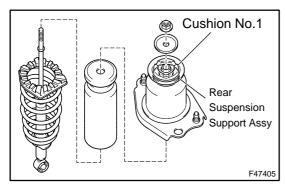
(e) Remove cushion washer No.1, cushion No.1, the rear spring front bracket, the rear suspension support assy, the rear coil spring insulator upper and rear spring bumper No.1.
