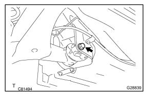
(b) Remove the 2 bolts and 2 nuts from the left– and right– hand sides.
