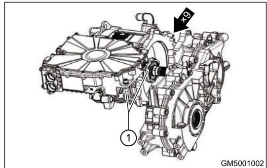
3. Remove motor output shaft from final drive input shaft.
