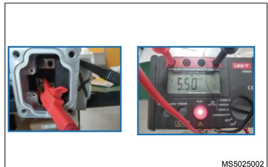
3. Connect the high voltage probe of insulation meter to the high voltage terminal of motor controller, and turn on the button to start the insulation test as shown in illustration. Use the same operation to test the high voltage DC bus input terminal of the motor controller, and record the test results.
