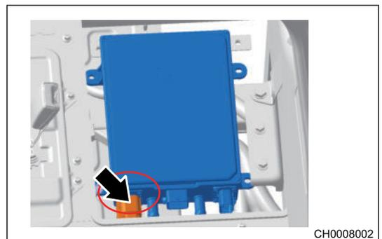
5. Remove the luggage compartment lower protector (arrow) (for removal procedure, refer to “Interior” and “Exterior” sections in “Body” ).
