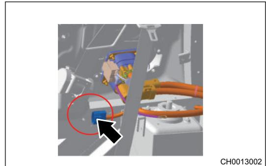
10. Remove 4 mounting bolts (arrow) from charging socket.
