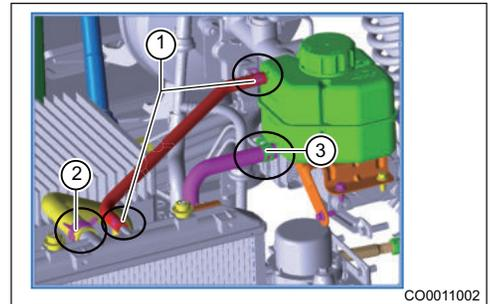
10. Gently break expansion tank clip to take out expansion tank, remove 3 fixing bolts (arrow) from expansion tank bracket with 6# socket, take out bracket.
