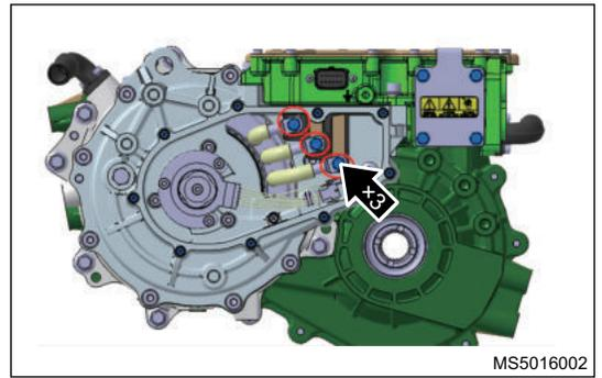
4. The removed drive motor controller is shown in illustration below.
