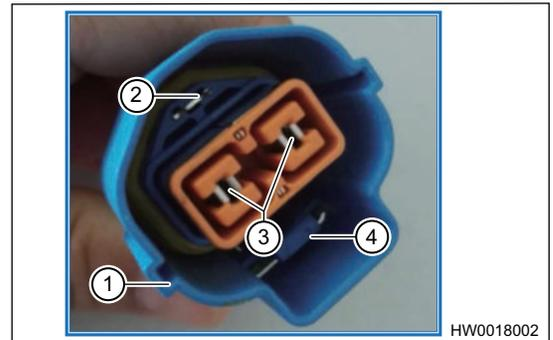
2. The connector is inserted in place, as shown in illustration below
