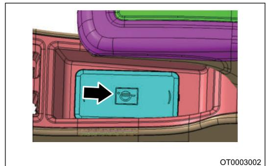
4. Press down and assemble wireless charging module in place.
