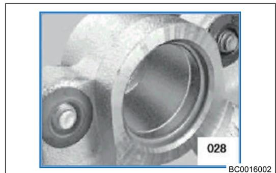
6. The area between dust seal ring and brake caliper housing must be kept dry. Do not allow to contact with brake cylinder grease or brake fluid to ensure the correct position of dust seal ring.
