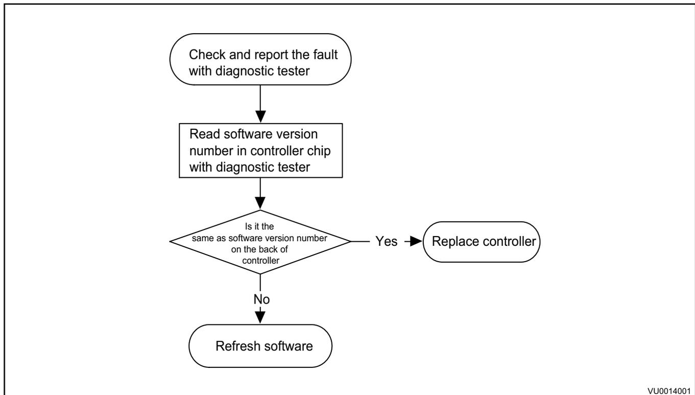
15. Motor System CAN Communication Receiving Failed U0293
