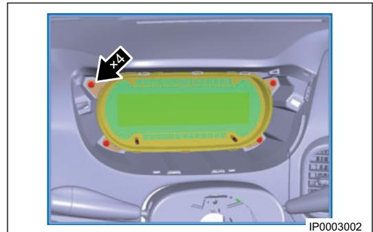
3. Disconnect instrument cluster wire harness connector, and remove instrument cluster.
