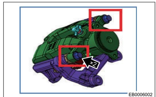
7. Remove the brake caliper body set.
