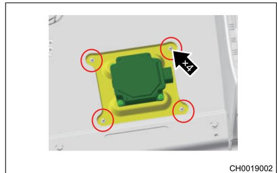
5. Remove the PLC communication module bracket.
