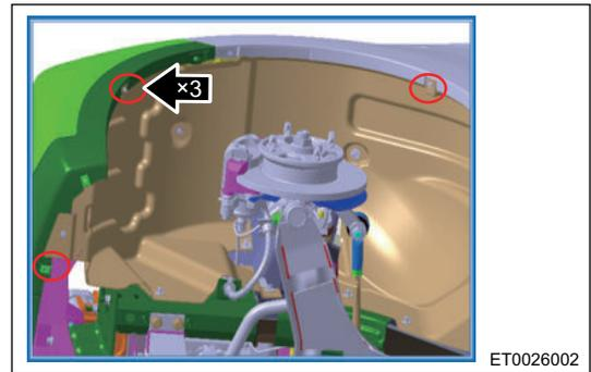
3. Using a cross screwdriver, remove 8 expansion clips (- arrow) from body, and remove front left wheel house protector.
