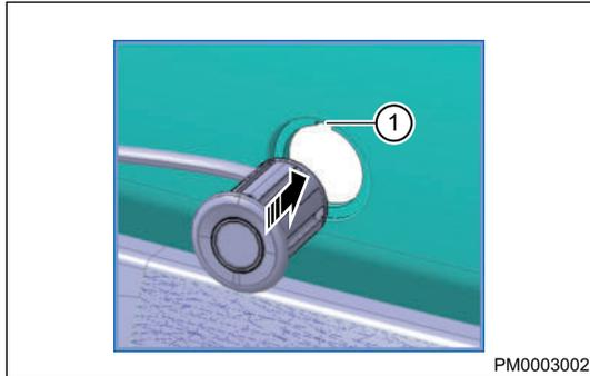
2. Connect sensor connector with indoor wire harness connector in place.
