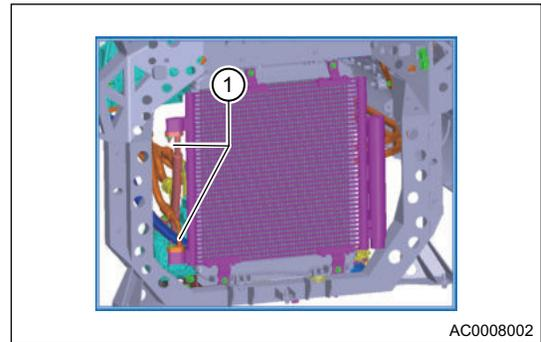
5. Remove 4 fixing bolts (arrow) from condenser and radiator assembly and condenser assembly.
