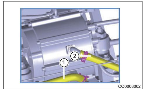
7. Remove clamp (arrow) between motor controller inlet pipe and floor cooling outlet pipe assembly.
