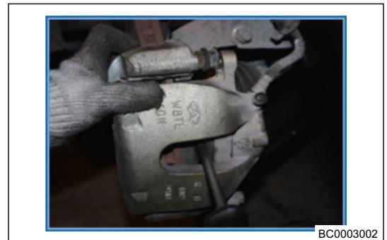
4. Remove caliper and brake lining, jam cylinder block with a filler (wood or foam) (1) and avoid piston sliding out.
