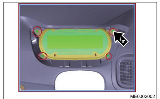
4. Disconnect the wire harness connector, and remove instrument cluster.
