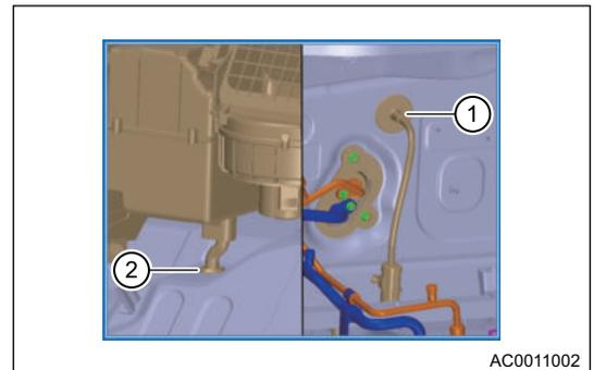
9. Remove 2 fixing nuts (arrow) from HVAC assembly at front compartment.
