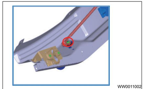
9. Remove 3 coupling bolts (arrow) between wiper motor and gutter channel, and remove wiper motor.
