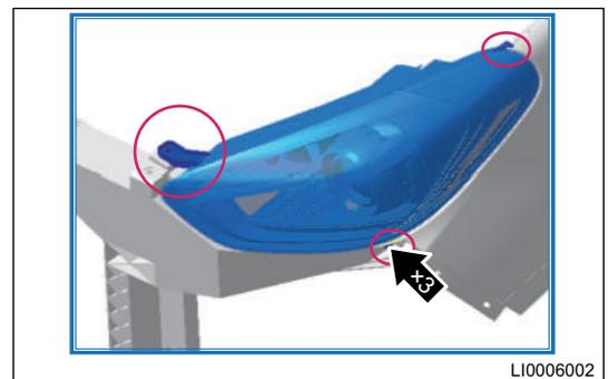
3. Disconnect wire harness connector from headlight and remove headlight assembly.
