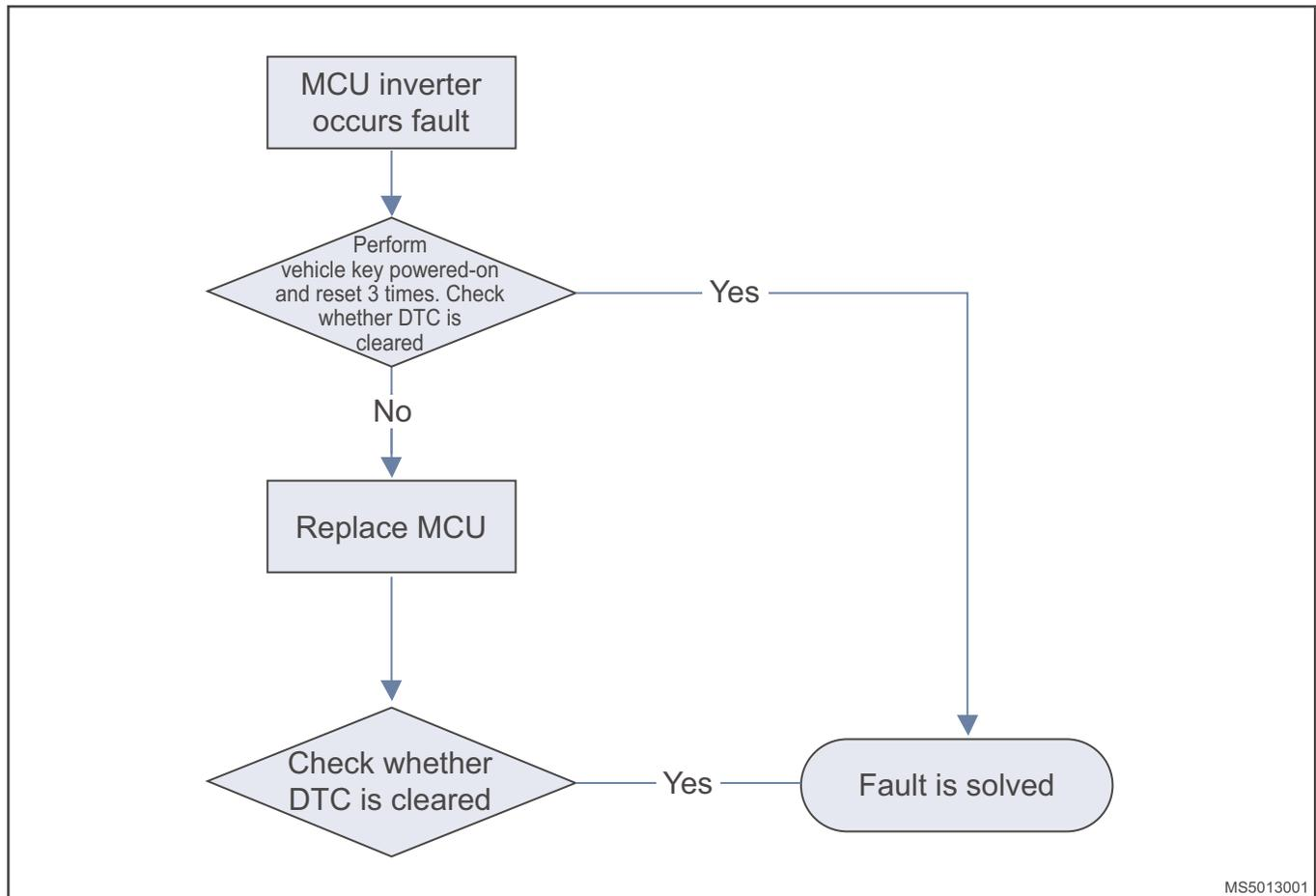
**DC Bus Overcurrent Fault P1A66**
