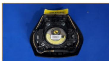
**Do not place end surface of airbag assembly downward**
