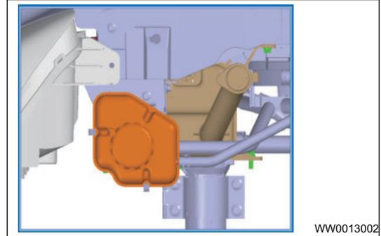
2. Disconnect connector and washer pipeline (arrow).
