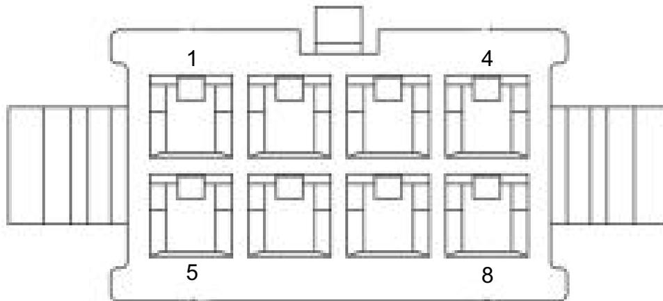
Motor Internal Resolver Signal Connector
