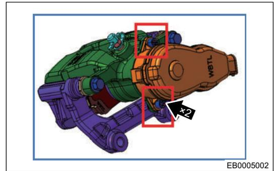
6. Remove fixing bolt (arrow) from brake caliper body with 13# socket.
