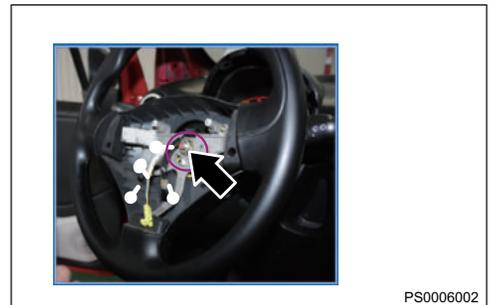
5. Using a cross screwdriver, remove 2 screws (arrow) from spiral cable, unplug wire harness connector, and remove the spiral cable.
