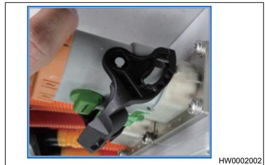
3. Separate connector from socket.
