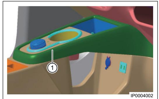
2. Using a flat tip screwdriver, pry off auxiliary fascia console rear end cover (1) assembly.
