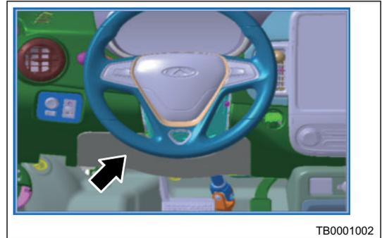
2. Disconnect the wire harness connector and combined antenna connector (arrow).
