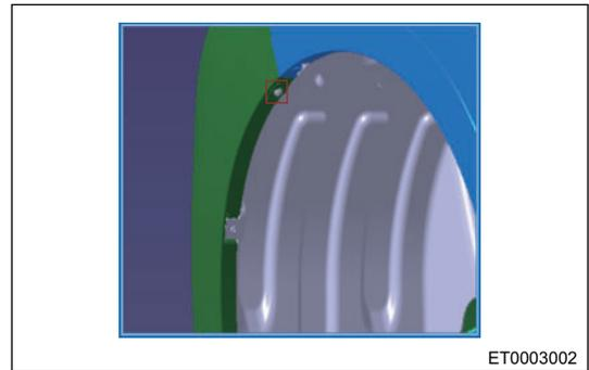
4. Using 8# socket wrench, remove 3 mounting bolts (arrow) from lower part of front bumper.
