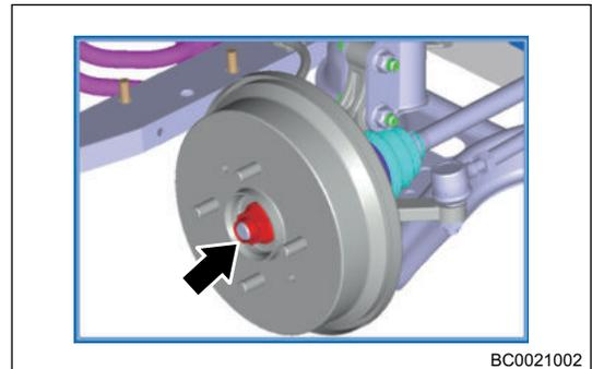
3. Remove the brake drum.
