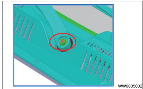
5. Remove sub wiper arm from installation position of output shaft (Removal steps of main wiper arm are the same).
