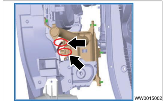
3. Loosen 4 mounting bolts (arrow) around reservoir, and remove the reservoir.
