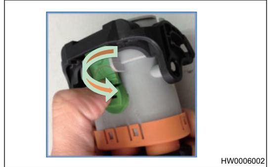
3. Insert connector into socket of battery pack.
