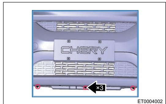
5. Using 8# socket wrench, remove 4 mounting bolts (arrow) from upper part of front bumper.
