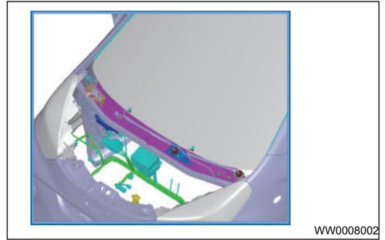
6. Remove the wiper output shaft trim.
