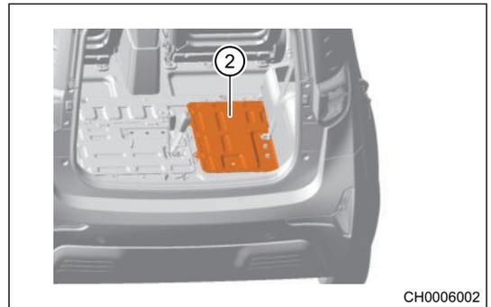
3. Remove the right quarter lower protector assembly (- arrow) (for removal procedure, refer to “Interior” and “Exterior” sections in “Body” ).
