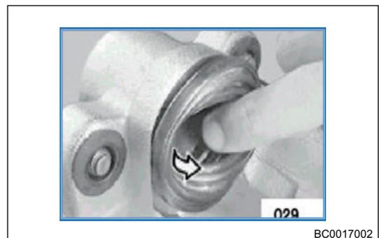
7. Brake piston is fixed with a extended part or a screwdriver and gently press it onto the dust seal ring. Blow the dust seal ring with compressed air (max 3.0 bar), install the piston ring on piston.
