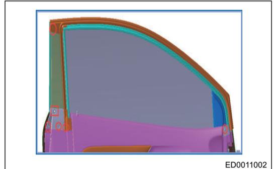
2. Using a cross screwdriver, remove clip and triangle protector (arrow) from door.
