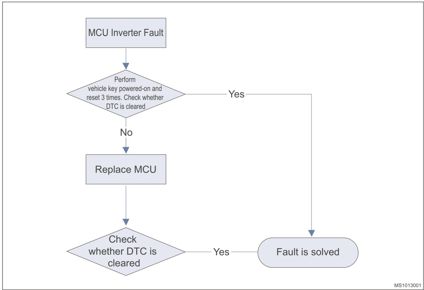
**DC Bus Overcurrent Fault P1A66**
