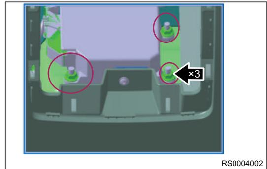
3. Unplug wire harness terminal connector, and remove airbag controller.
