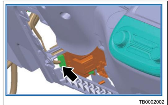
3. Remove 2 fixing bolts (arrow) from diagnosis device, and remove diagnosis device assembly.
