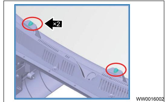
2. Disconnect the washer pipeline (arrow), and remove washer nozzle.
