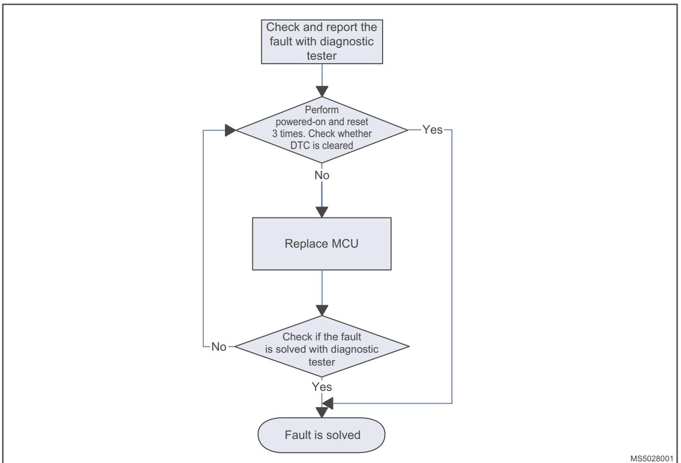
**MCU Hardware Latch Fault P0A55**
