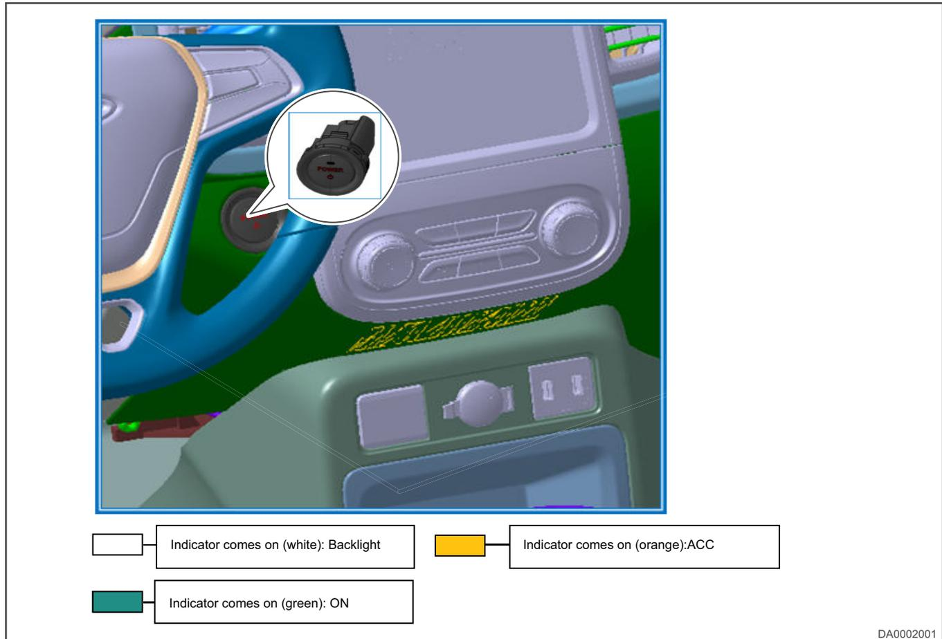
POWER switch is installed in a prominent position on instrument cluster, providing the BCM controller with the transition of vehicle power supply state and the input signal controlled by VCU.
