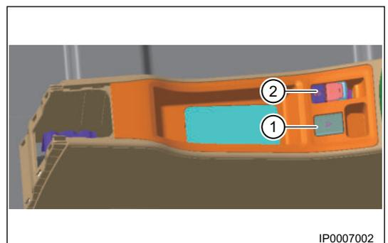
4. Pull parking brake lever to the upper limit position. Using a flat tip screwdriver, pry off accessories such as parking brake cover plate assembly, warning light switch (1), automatic parking switch (2), and then unplug wire harness connector on back (for models without armrest).
