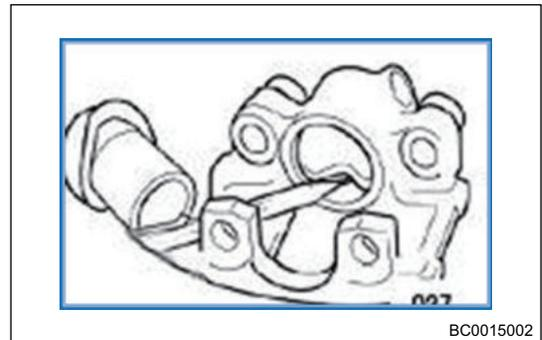
5. (Installation of brake wheel cylinder) apply a thin film of brake cylinder grease on cylinder block, plunger and sealing boot. Install seal ring in the rear ring groove of brake cylinder. Install dust seal ring in the front ring groove and press it fully.
