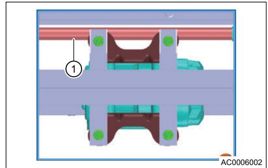
6. Remove 4 fixing bolts (arrow) from compressor bracket and A/C compressor assembly with bracket.
