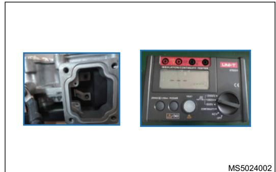
2. Connect the ground wire of insulation meter to the housing of the motor controller at the position indicated by the black clip as shown in illustration.
