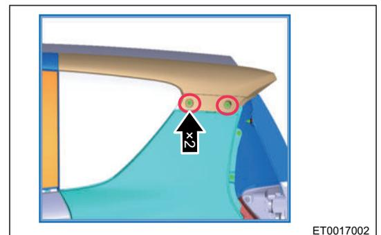
3. Using a flat tip screwdriver, carefully pry off and remove the left top side beam outer panel rear trim panel assembly.
