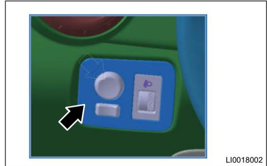
2. Press and hold the clip to remove the headlight leveling switch.
