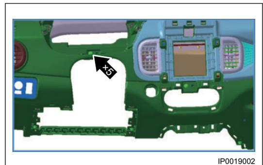
12. Remove the instrument panel assembly.
