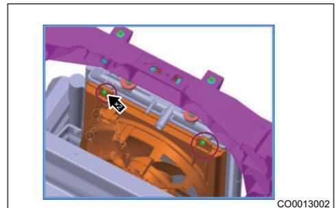
12. Remove front bumper assembly, front bumper lower protector, front bumper crossmember assembly (refer to "Interior" and "Exterior" sections in "Body").
