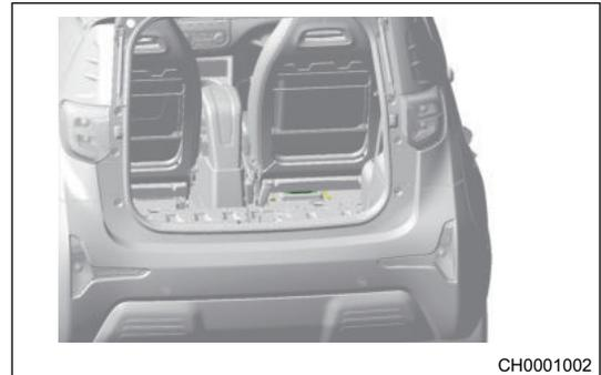
2. Remove 2 rear service hole cover plate assemblies 1 and 2 as shown in the illustration (for removal procedure, refer to “Interior” and “Exterior” sections in “Body” ).
