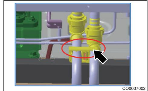
6. Remove clamp between motor outlet pipe and floor cooling outlet pipe assembly, drain motor coolant (1 is motor inlet pipe, 2 is motor outlet pipe).
