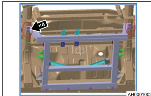
2. Using 15# socket and torque wrench, remove 4 tightening bolts (arrow) from rear part of front sub frame and front sub frame.
