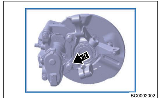
3. Pry the brake wheel cylinder with a flat tip screwdriver.
