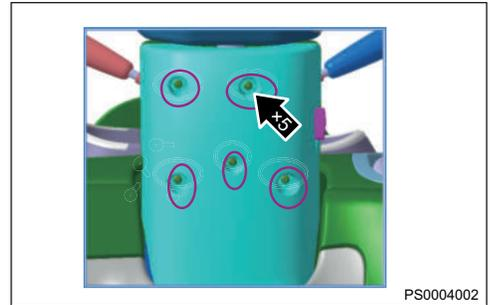
3. Using a flat tip screwdriver, jack up preload spring (arrow) of upper cover, and remove driver airbag.
