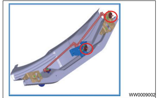
7. Remove 6 mounting nuts between wiper output shaft and bracket.
