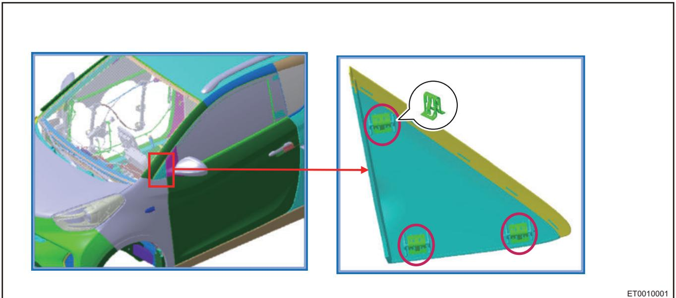
1. Using a flat tip screwdriver, pry from near the three mounting points of front left quarter triangular block in the order of 1-2-3, pry off mounting points from three corners. A soft material such as foam should be placed under screwdriver to prevent wing from being scratched.
