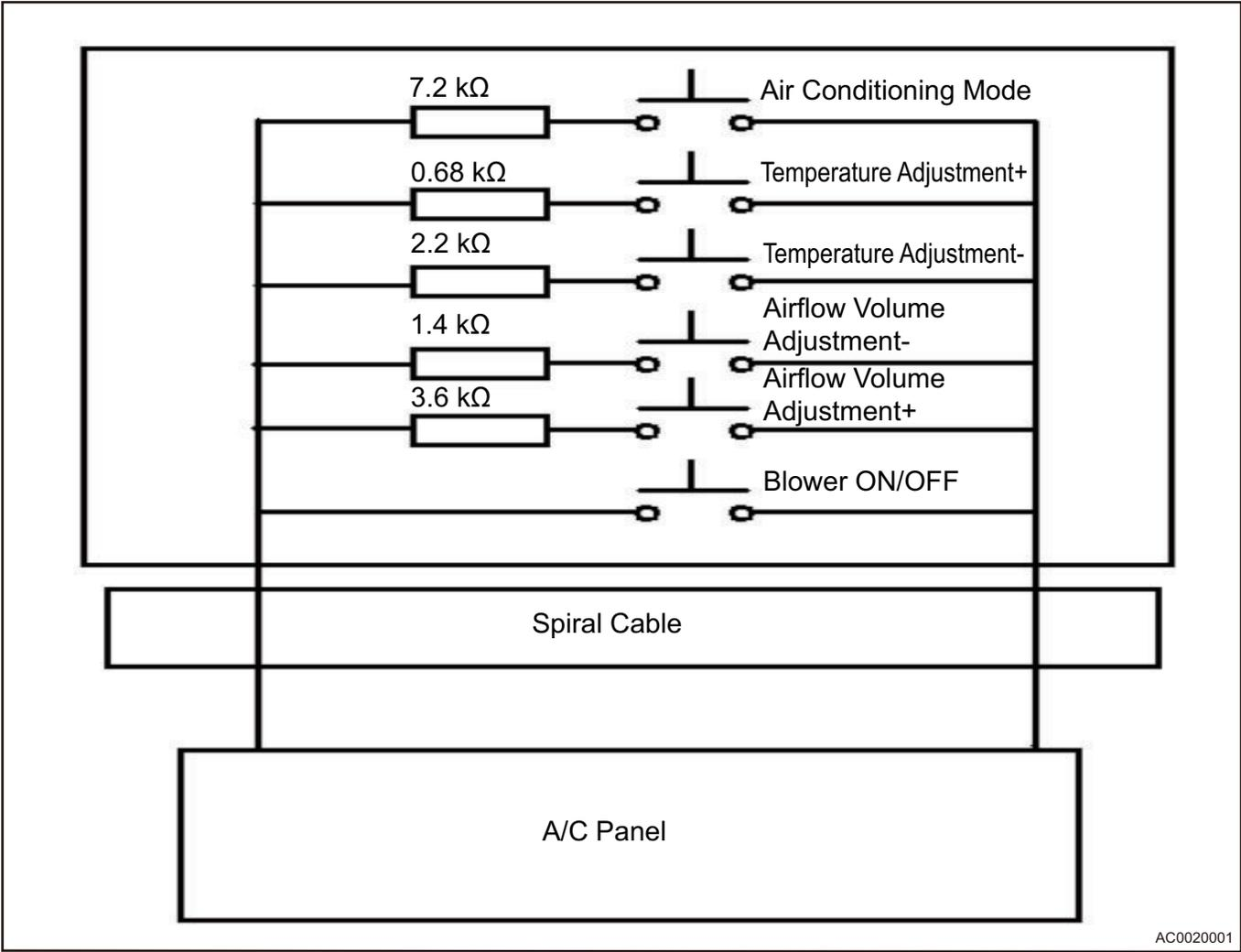
**A/C Pressure Switch Circuit Schematic Diagram**
