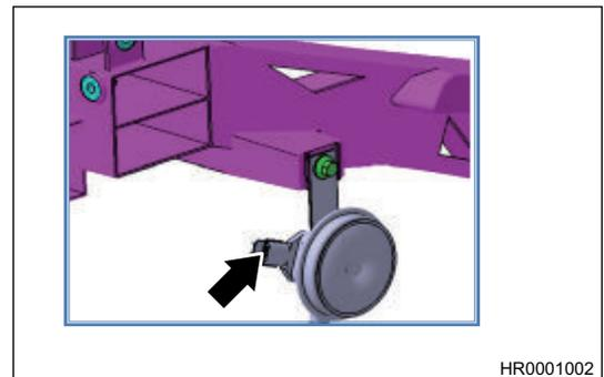
4. Remove the high pitched horn fixing nut (arrow) with 13# socket.
