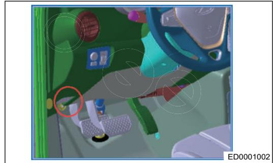
2. Operate front compartment cover lock safety hook handle to fully separate upper and lower parts of front compartment cover lock, then pull out rear pin of front compartment cover assembly from mounting bracket.
