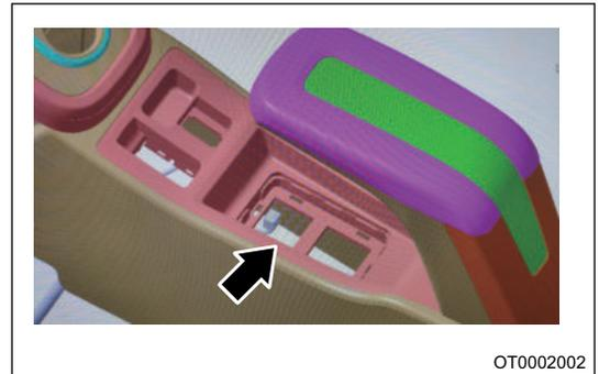
2. Connect the wireless charging module connector properly.
