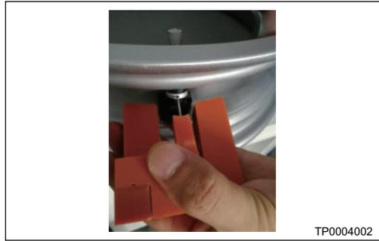
5. Using a electric gun (or torque wrench), tighten the nut, and keep the sensor gum application surface facing the rim surface after tightening (it can be deflected slightly).
