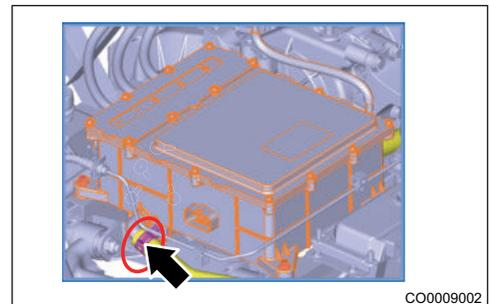
8. Unplug fixing clips (arrow) from rear compartment cooling pipe assembly.
