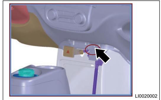
3. Remove the hazard warning light switch.
