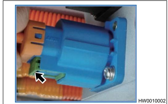
2. Press blue buckle (1) once and pull out connector. After pulling out connector, pay attention to lock green pull ring (2).
