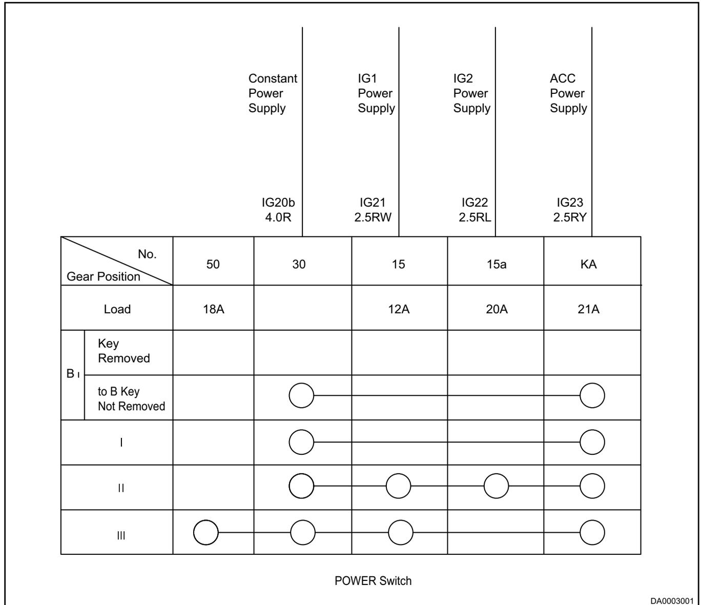
POWER Switch has four gear positions: LOCK ← ACC ← ON ← START. In LOCK position, the locking tab pops out to lock the steering column and prevent from rotation, and in other positions, the locking tab is retracted, and the steering column can be rotated. After releasing from START position, the key will automatically return to ON position. If you want to change from ACC to LOCK, you need to press the switch and then turn to LOCK position.
