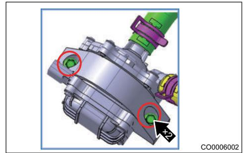
5. Remove water pipe connector and pull out water pipe fixing clip (arrow).
