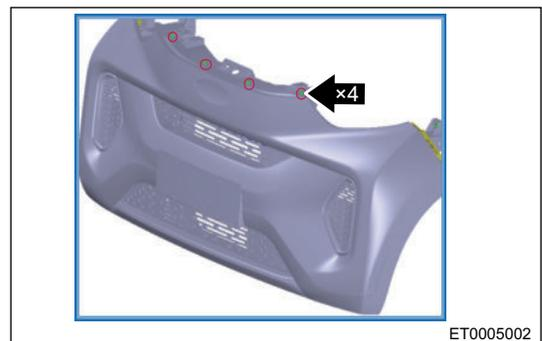
6. Pull out left/right side of front bumper from front bumper mounting bracket clips.
