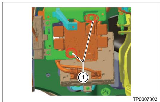
3. Remove 5 connectors (1) from body control module.
