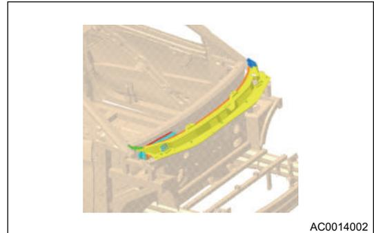
2. Using a socket, remove 2 nuts, and remove element and its mounting bracket.
