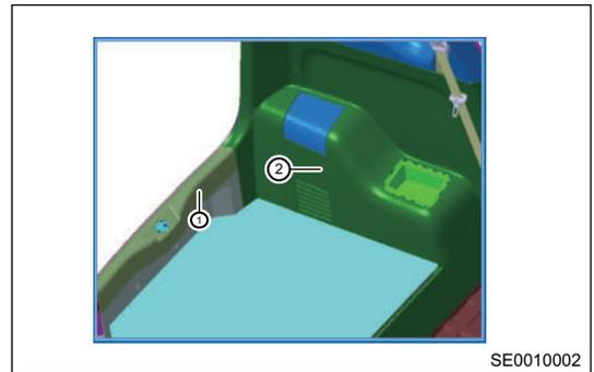
2. Using torque wrench and 17# socket, loose seat belt bolt (1).
