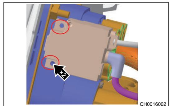
4. Remove the charging port electronic lock.
