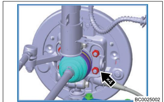
7. Remove the hub bearing unit assembly.
