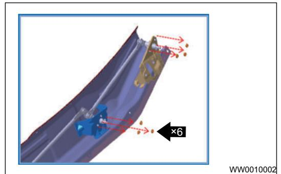
8. Remove coupling nut between wiper connecting rod crank and wiper motor output shaft with torque wrench, and remove wiper link rod assembly.
