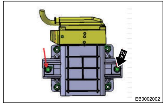
4. Remove EPB controller from auxiliary fascia console quarter.
