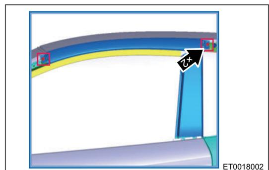
3. Using a flat tip screwdriver, carefully pry off and remove the left top side beam outer panel front trim panel assembly.
