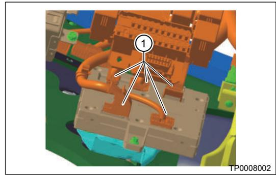
4. Remove 3 M6 fixing bolts (arrow) from body control module, and body control module can be removed.
