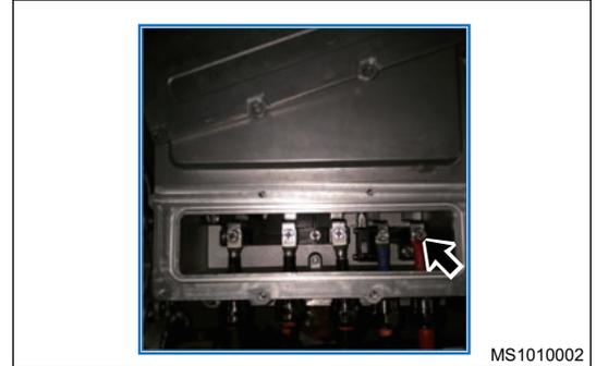
2. Use a multimeter to detect the resistance between phase A and phase B, phase B and phase C, phase A and phase C of the motor to check whether there is phase loss. It is determined that motor is missing phase if the difference between them is more than 0.5  $\Omega$ . Please replace the motor.
