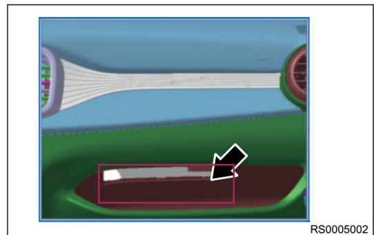
2. Unscrew front passenger airbag fixing bolt from glove box PAB inspection and repair cover plate.
