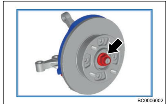
7. Remove front hub and then remove brake disc.
