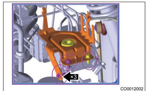
11. Using 6# socket, remove mounting bolt (arrow) from electronic fan, unplug fan connector, take out the fan.
