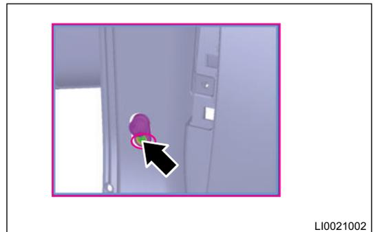
2. Disconnect the connector and remove the rear door contact switch.
