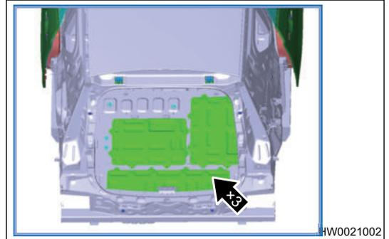
2. Use inner hexagon wrench to remove upper cover bolts (- arrow) from junction box.
