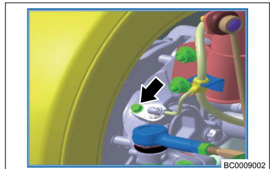
10. Remove 2 nuts (arrow) between shock absorber and steering knuckle with pneumatic wrench and 18# socket.
