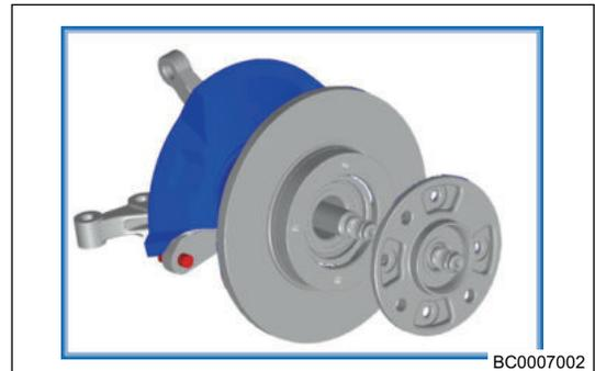
8. Remove coupling nut (arrow) between brake fluid pipe and brake wheel cylinder with 13# speed wrench and save 2 shims. Recycle brake fluid in a clean container and then remove brake wheel cylinder (if only replace brake disc, it is not required to disconnect brake line.)
