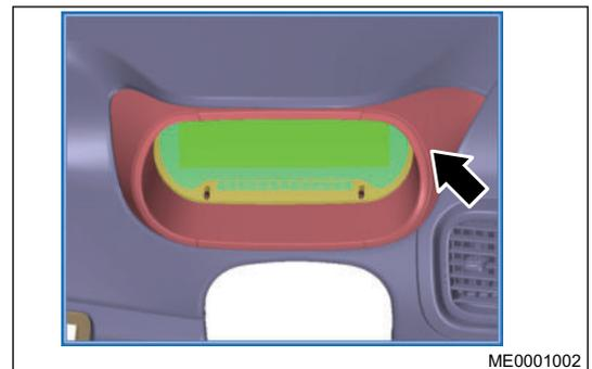
3. Remove fixing screws (arrow) between instrument cluster and instrument panel with a cross screwdriver.
