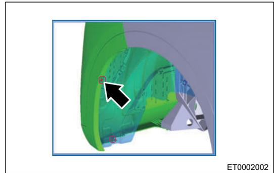
3. Using a cross screwdriver, remove mounting screw from front bumper (both sides) and front bumper mounting bracket.
