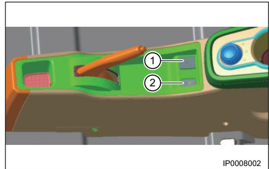
5. Remove the auxiliary fascia console assembly.
