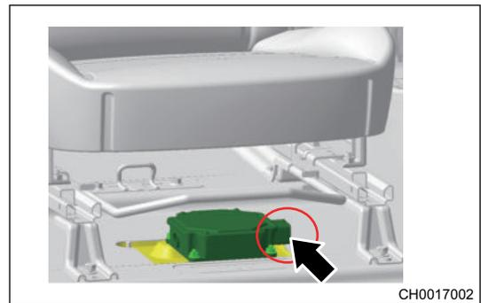
2. Remove 4 mounting nuts (arrow) from PLC communication module.
