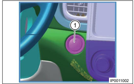
5. Remove the left lower switch control panel. Using a flat tip screwdriver, pry off left lower switch cover plate, then disconnect wire harness connector to remove left lower switch cover plate.
