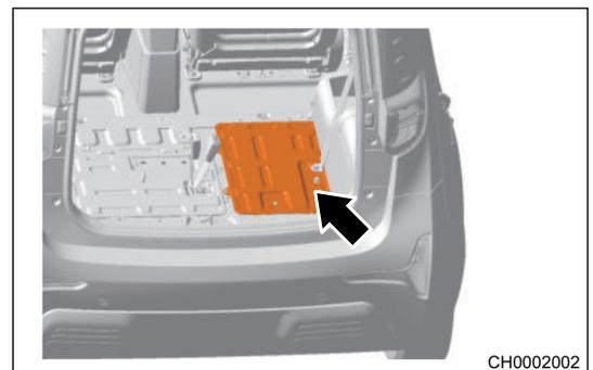
3. Unplug all connectors, pipes and ground that are connected to on-board charger DCDC converter assembly.
