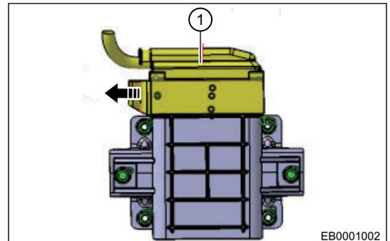
4. Using 8# socket, remove 1 fixing bolt (arrow) from rear left wheel speed sensor and wheel speed sensor.
