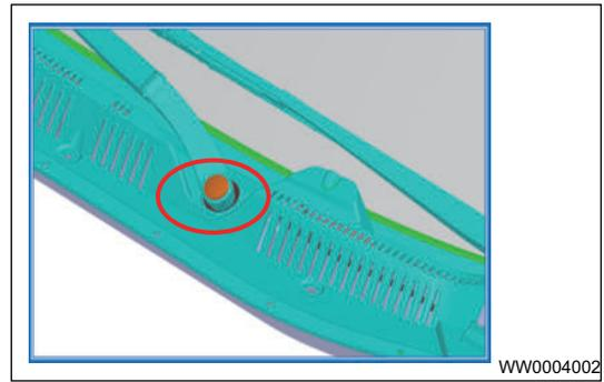
4. Remove mounting nut between sub wiper arm and output shaft with torque wrench and socket 13#. Tightening torque:  $18 \pm 2$  N·m
