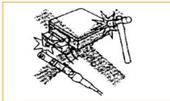
**Do not hit controller with wrench or hammer**
