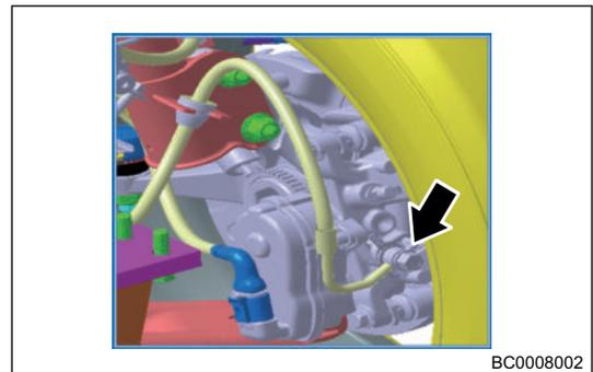
9. Remove 1 M6 fixing bolt (arrow) from front wheel speed sensor with 8# speed wrench, remove connector from wheel speed sensor.
