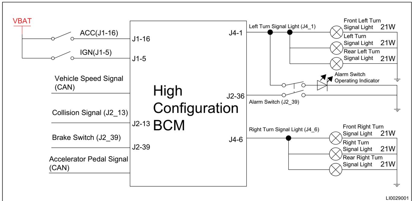
**Sudden Braking Flashing Function Description**
