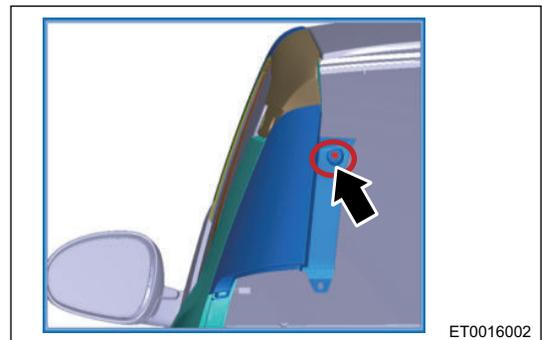
3. Using a flat tip screwdriver, carefully pry off rear left quarter ornament assembly (for clip position, refer to composition diagram of mounting points).
