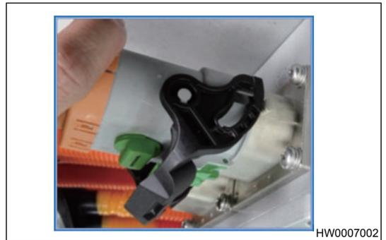
4. Insert connector with force and toggle handle until a click is heard to indicate that it is assembled in place.
