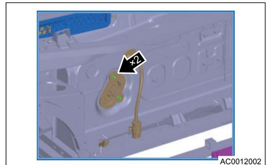
10. Remove 7 fixing bolts from HVAC assembly in passenger compartment to remove HVAC assembly.
