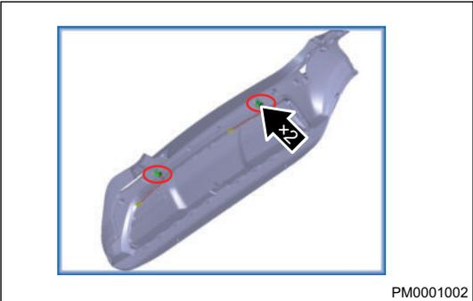
3. Using a flat tip screwdriver, unscrew clamping reed, and remove reverse radar sensor.
