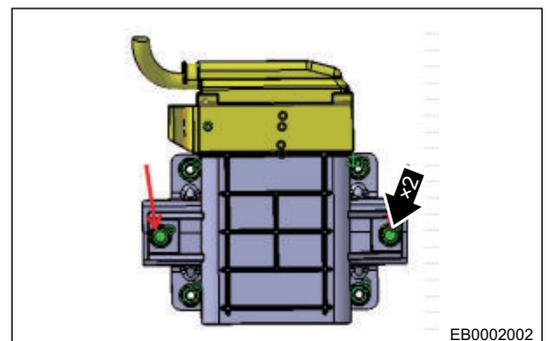
5. Remove fixing nut from rear axle left drive shaft.
