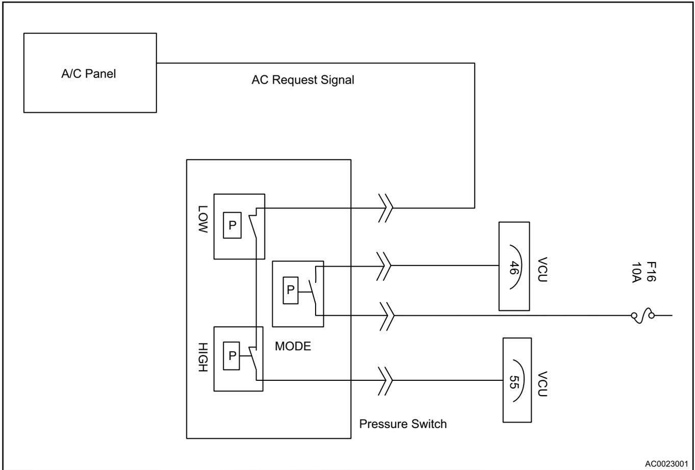
**Refrigerant System Circuit Schematic Diagram**
