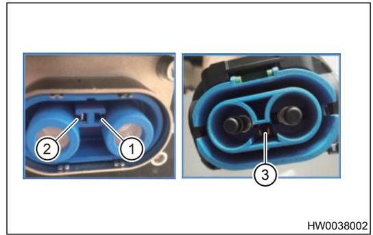
2. Repair method of faulty area ①.
