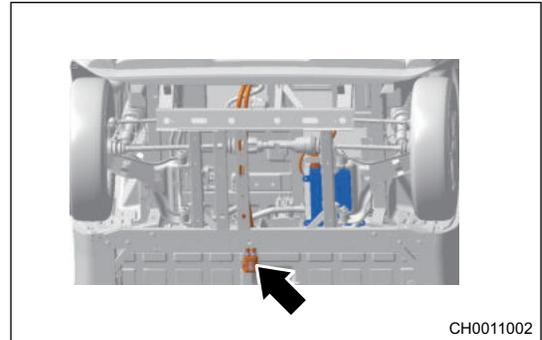
8. Remove charging port wire harness boot, clip on each position and ground bolts.
