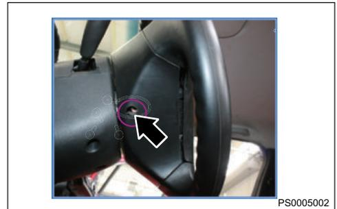
4. Remove steering wheel nut (arrow) with 22# socket and ratchet wrench, and remove the steering wheel.
