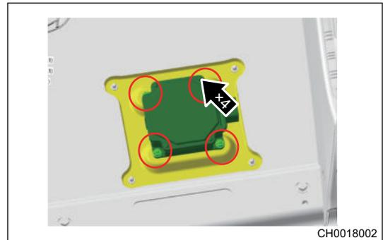
3. Remove the PLC communication module.
