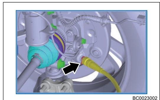
5. Remove 1 M6 fixing bolt (arrow) from front wheel speed sensor with 8# speed wrench, remove connector from wheel speed sensor.
