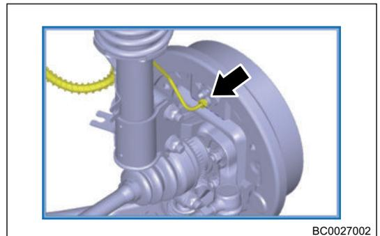
9. Remove 2 nuts (arrow) between shock absorber and steering knuckle with pneumatic wrench and 18# socket.
