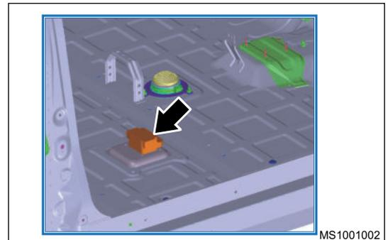
2. Remove rear service port cover plate assembly (arrow).
