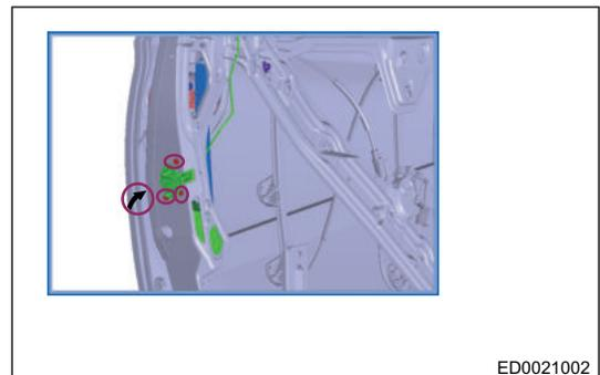
3. Using a cross wrench, remove 3 fixing screws from door lock, and remove door lock assembly.
