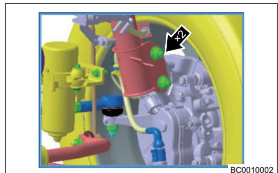
11. Remove 1 nut (1) between steering tie rod and steering knuckle with pneumatic wrench and 19# socket, and then remove 1 bolt (2) between swing arm and steering knuckle with pneumatic wrench and 18# socket, finally remove front steering knuckle.
