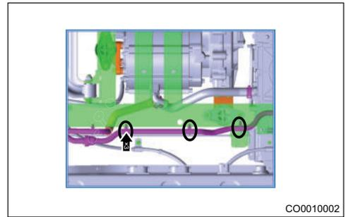
9. Lower the vehicle and remove radiator discharge pipe clamps (both sides), radiator inlet hose clamp and expansion tank outlet pipe (1 is radiator discharge pipe, 2 is radiator inlet hose, 3 is expansion tank outlet pipe).
