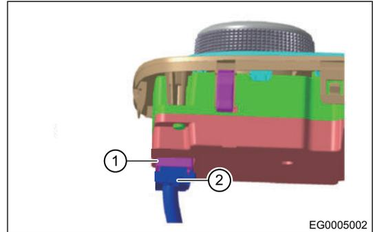
3. After connectors are connected in place, clamp automatic shift control mechanism assembly and shift panel as a whole into auxiliary fascia console (1) (clamp from top to bottom in a direction perpendicular to auxiliary fascia console).
