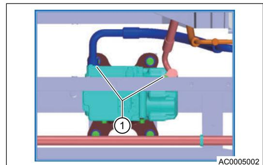
5. Remove the front suspension lateral stabilizer bar (1).
