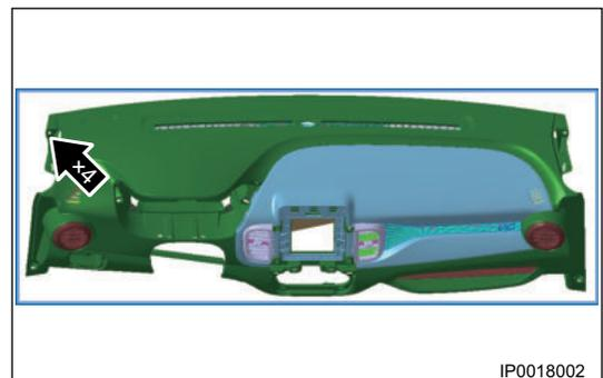
11. Remove 5 fixing screws (arrow) between instrument panel and instrument panel crossmember.
