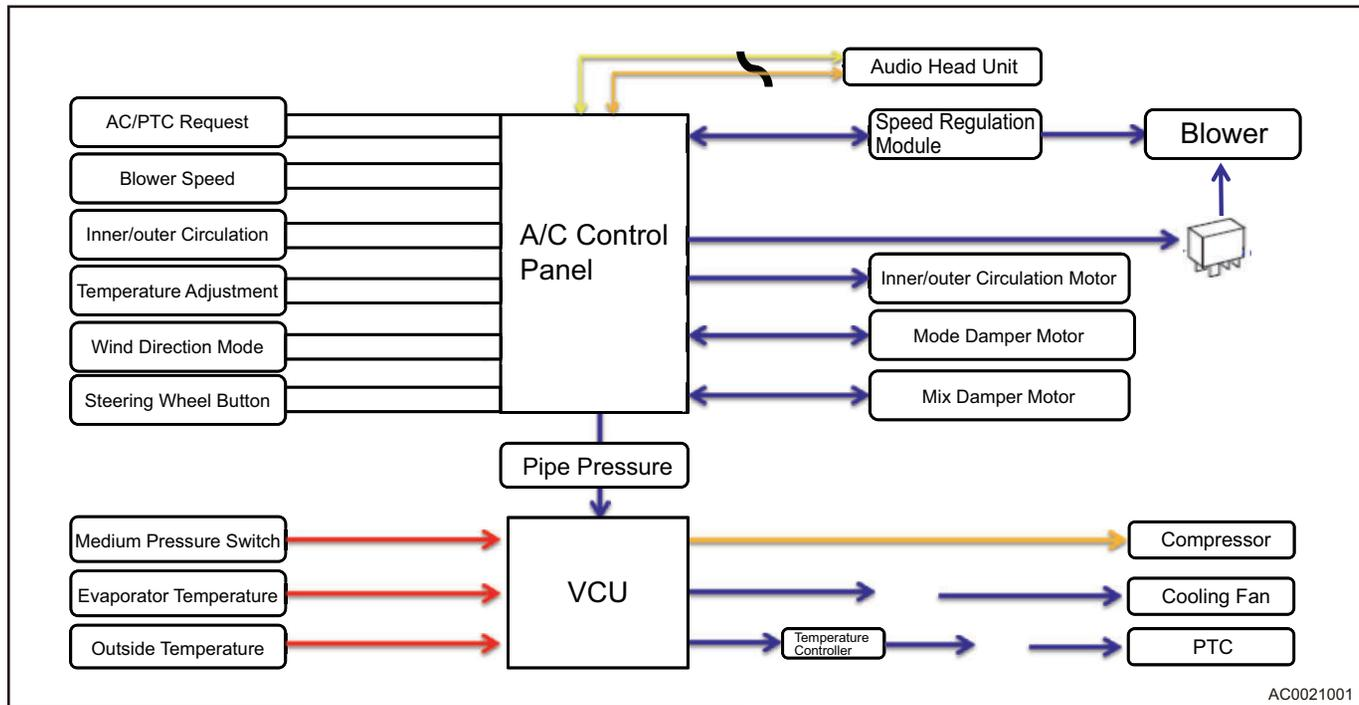
Refrigerant System Schematic Diagram
