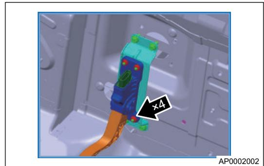
5. Unscrew 4 fixing bolts (arrow) from electronic accelerator pedal mounting bracket with 10# socket, and remove bracket.
