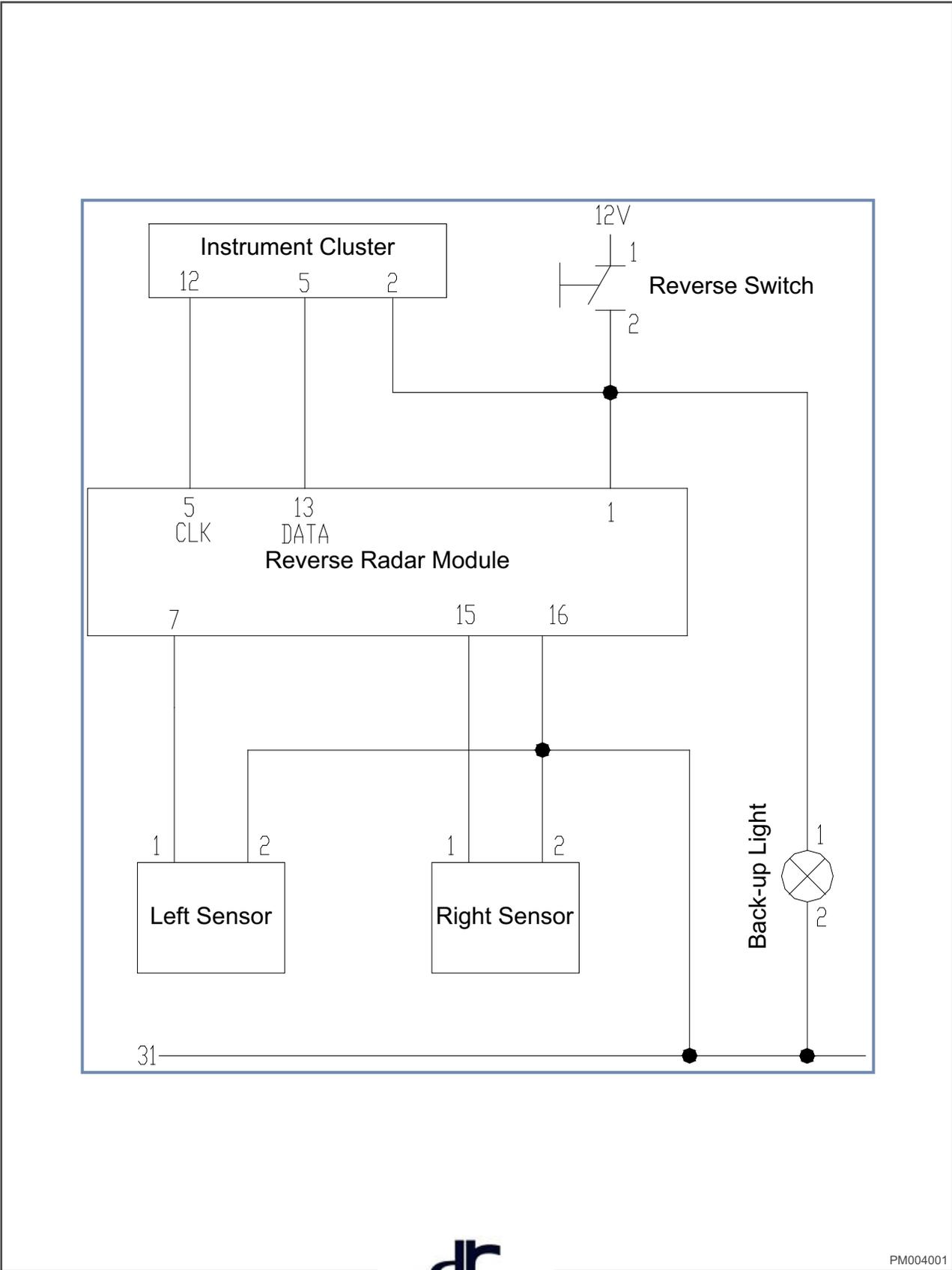
**Reverse Radar Module Pin Definition**
