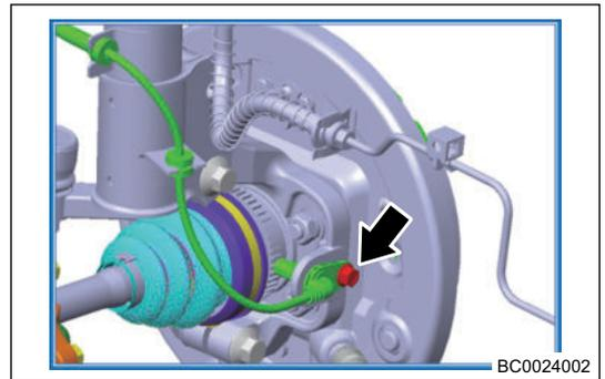
6. Remove 4 fixing nuts (arrow) from steering knuckle and hub bearing unit assembly with 16# socket and pneumatic wrench.
