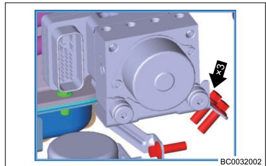
4. Remove 3 bolts (arrow) between controller and bracket with inner hexagon wrench.
