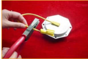
**Do not cut wire or damage connector terminal**
