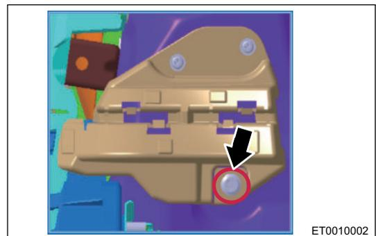
3. Using a cross screwdriver, remove 2 upper cross-recessed button head self-tapping screws and rear bumper left/right mounting bracket.
