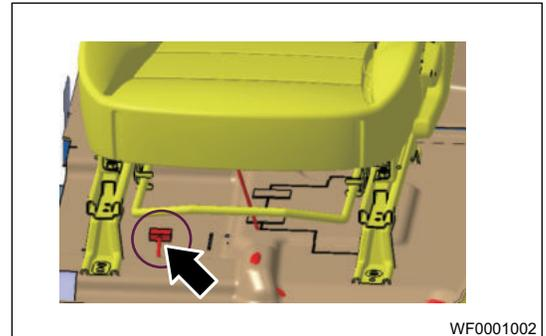
3. Firmly connect the Wifi module wire harness connector with the product end connector.
