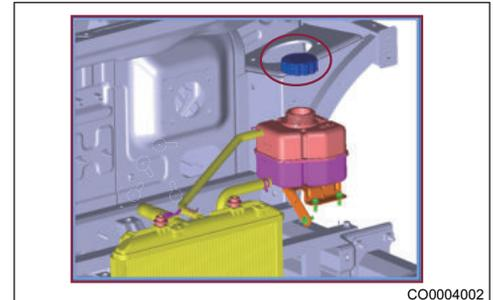
3. Prepare an antifreeze collection bucket, loose clamps (- arrow) from water pump inlet and outlet pipe assembly with clamp plier, and drain coolant.
