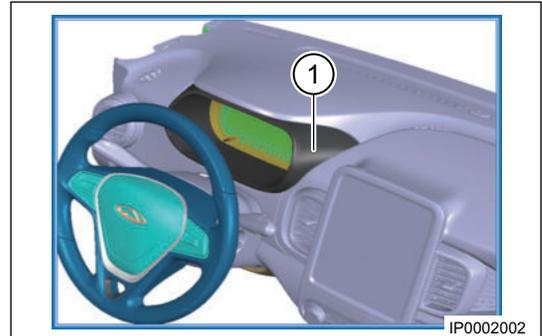
2. Using a cross screwdriver, remove 4 fixing screws (arrow) between instrument cluster and instrument panel.
