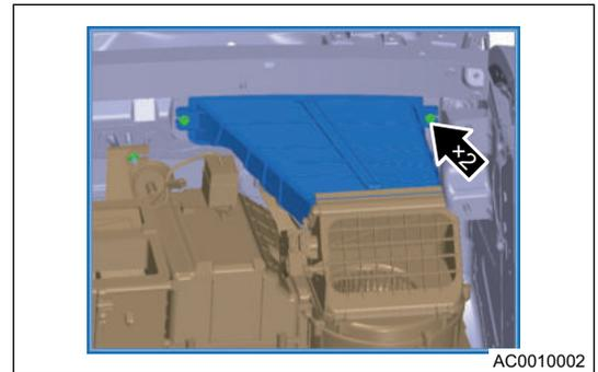
8. Remove PTC wire harness seal rubber sleeve (1) and seal rubber sleeve from drain pipe (2), and push PTC wire harness on HVAC to passenger compartment.
