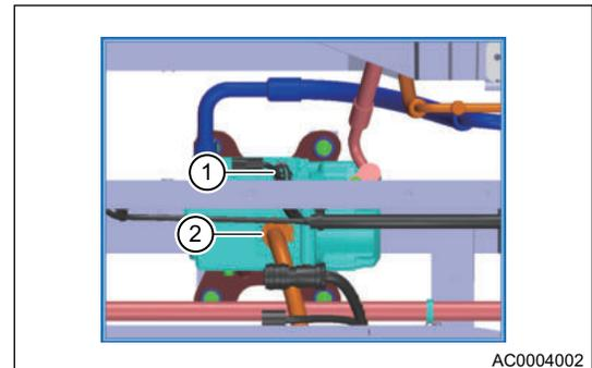
3. Drain the refrigerant in A/C.
