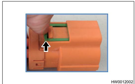
2. Insert wire harness connector into socket, press connector firmly until a click is heard to indicate that it is assembled in place.
