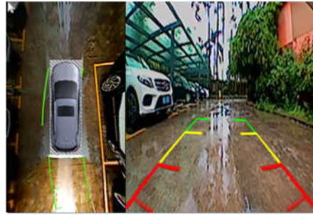
The reflective effect of accumulated water on rainy days is poor
