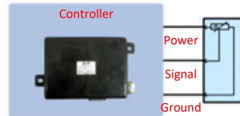
Sensor Power Circuit ≠ Sensor Signal Circuit
