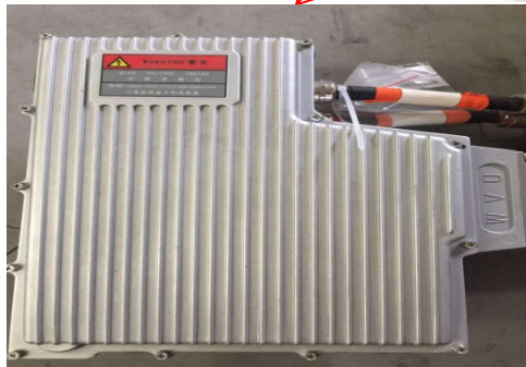
Drive Motor Controller
