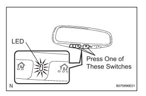
(b) Erase the transmitter codes in the garage door opener clear mode.
