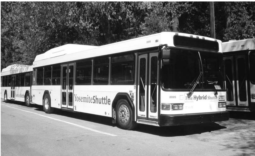
FIGURE 3.2 Free Yosemite hybrid shuttle, a gillig bus with GMC hybrid propulsion. (Photograph by the author in Yosemite National Park, 30 April, 2007.)
