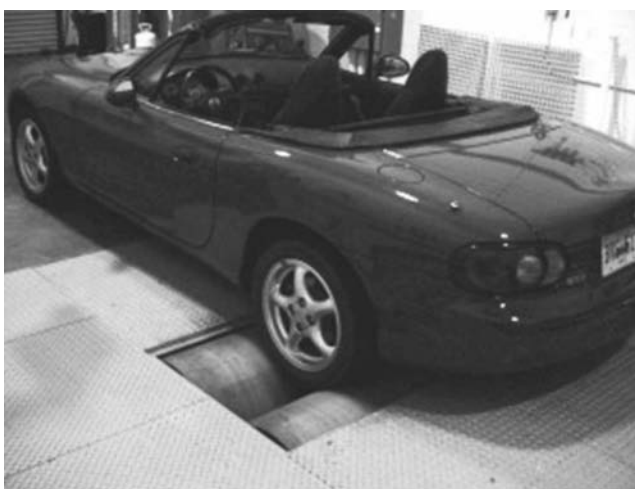
FIGURE 12.2 Vehicle positioned on a dynamometer in an EPA test facility. Tests for fuel economy and emissions are conducted. Note the two rollers for the dynamometer. The two rear drive wheels are on the rollers. (Reproduced from Environmental Protection Agency. Available at www.fueleconomy.gov/feg/fe_test_schedules.shtml .)
