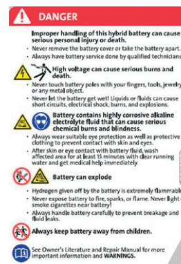
Warning label sticker on the high voltage battery
