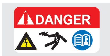
Warning label sticker on the high voltage components
