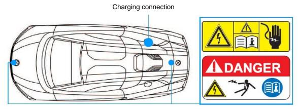
High-voltage warning signs under the bonnet and under the boot lid
